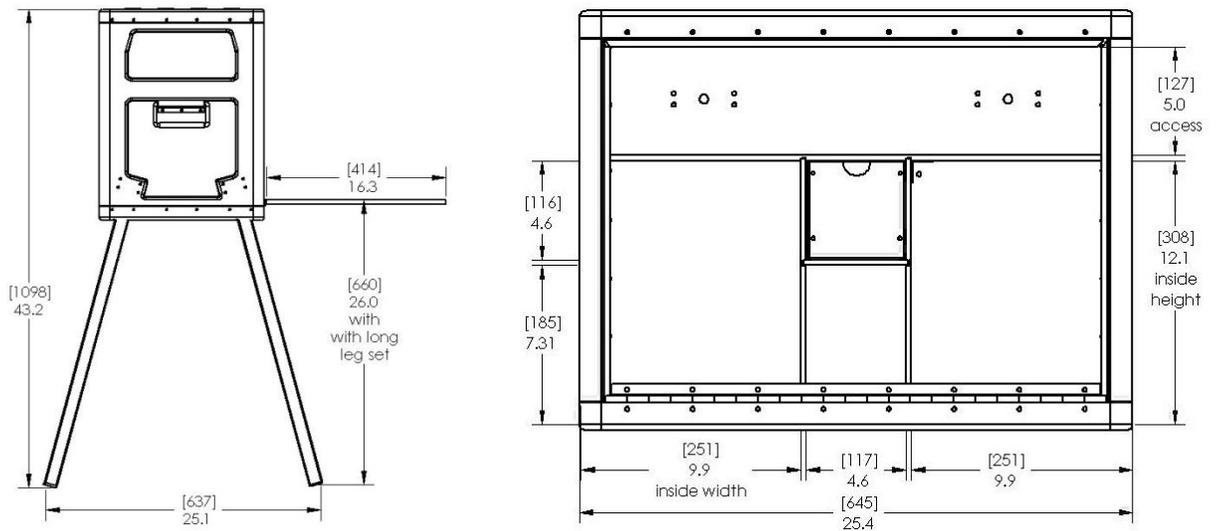
*Side view with optional long leg set (subtract [152 mm] 6.0 inches in height for short leg set)*
